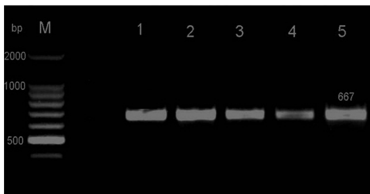
Fig. 1 -Agarose gel of HSP70h PCR products. M Marker (100 bp ladder), lane 0 negative control, lane 1 positive control, lane 2 KP243751, lane 3 KP243759, lane 4 KP243752, lane 5 KP243754. Bands correspond to amplicons having a size of 667 bp.
